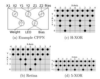
Figure 1: Example CPPN and geometric layouts. (a) A CPPN example (see section 2.1). (b) Geometric layout for the Retina Problem. (c) Geometric layout for the H-XOR problem. (d) Geometric layout for the 5-XOR problem. Note that, the z coordinates of all nodes are 0.
