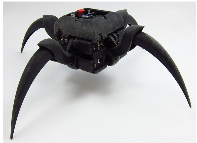
Figure 1: Aracna: an open-source 3D printed quadruped robot platform, here printed in a black rapid prototyping polymer. STL files for 3D printing the robot and drivers for the Arbotix board and servos are publicly available at http://creativemachines.cornell.edu/aracna .
