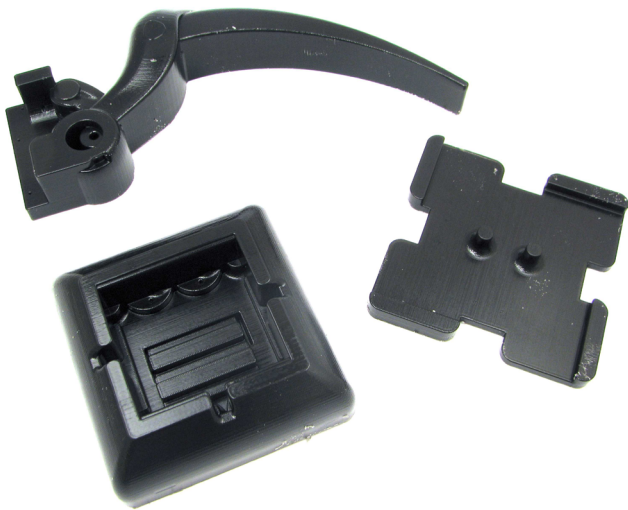
Figure 6: A final version of Aracna printed in multiple pieces. The body is printed as two pieces, with 9 smaller parts within the top piece to reduce support material and print time. These parts can be printed individually if replacements are necessary. The body consists of a total of 11 parts. This image shows a set of 12 printed parts (the complete body and a single leg) with support material still present.
